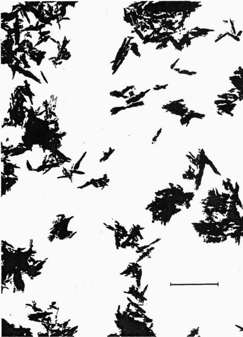
Fig. 1. Transmission electron micrograph of hydroxyapatite powder. Note the elongated shape of the primary particles. Although isolated particles are observed, most of them are aggregated. Scale bar is 0.5 \mu\text{m} .
